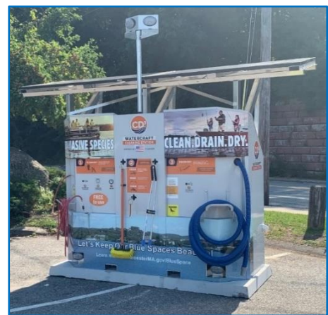
Figure 12 - Solar powered boat decontamination stations were installed at Indian Lake and Coes Reservoir to enable lake goers to decontaminate their watercraft before and after use to avoid transporting invasive plants to the lakes.
